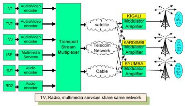
Fig. 3: The digital terrestrial broadcasting principle
